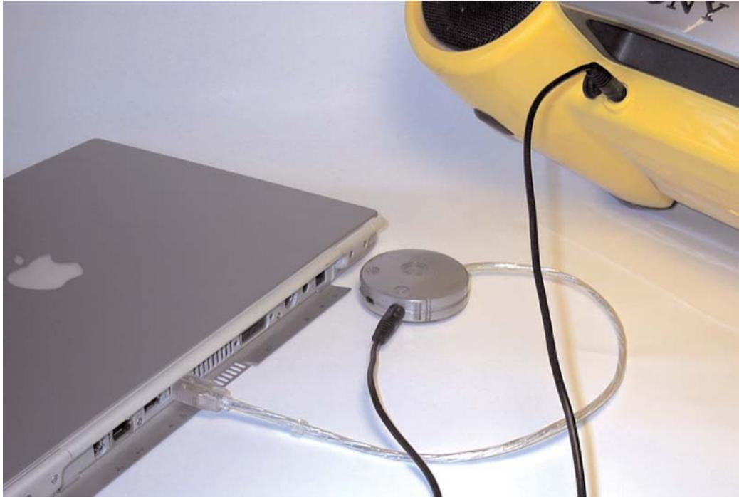
Fig. 89 – Macintosh computers that do not feature built-in sound input will need to use some type of audio interface – the Griffin iMic is shown above, plugged into a USB port. The audio output from the stereo equipment feeds into the audio input of the iMic, then into the com-
