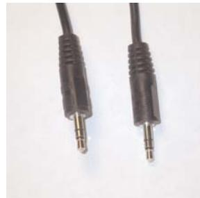
Fig. 86 – The cable used to connect these two devices together has a 1/8" stereo connector at both ends
