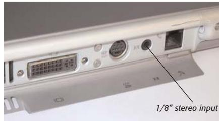
Fig. 11 – The built-in audio input on an 800MHz Titanium Powerbook
