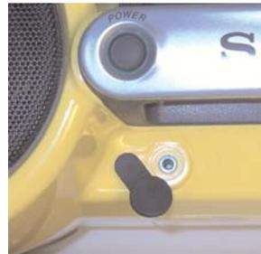
Fig. 7 – As this cassette player has only a 1/8" headphone output, we'll use this to connect to the Mac's built-in audio input.
