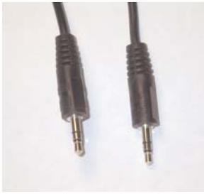
Fig. 84 – The cable you need to use in this configuration has this type of connection (1/8" mini-plug) at both ends.
