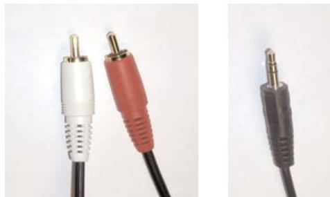
Fig. 88 – The cable used to connect a cassette player to an Edirol UA1A has a 1/8" stereo connector on one end and RCA connectors on the other end.
