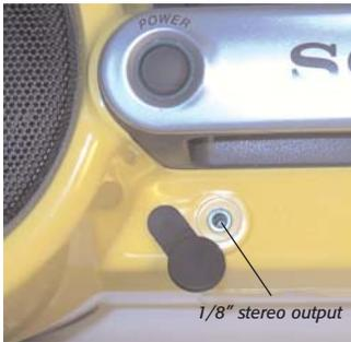
Fig. 9 – Example of a 1/8" stereo headphone output on a cassette player
