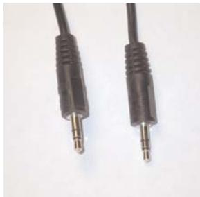
Fig. 10 – The cable used to connect these two devices has a 1/8" stereo connector at both ends
